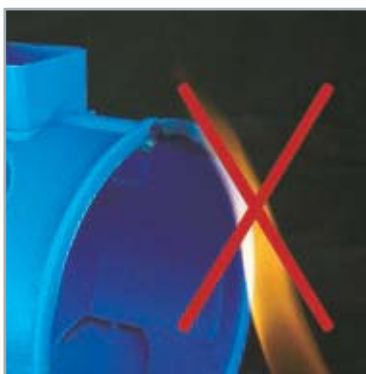
Tworzywo samogasnące poliamid PA 6 Self-extinguishing polyamide PA 6
