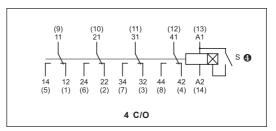
Ontrol contact S is activated by connecting it to A1 terminal.
