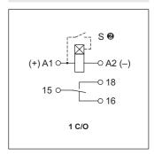
**②** Control contact S is activated by connecting it to A1 terminal.
